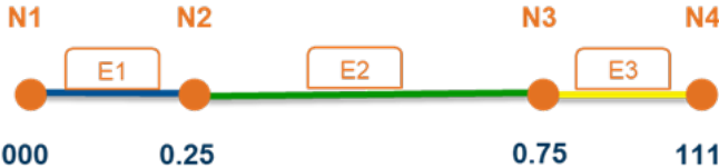
Figure 42: 1D IGA element based on open knot vector
